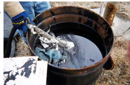
Thick, viscous tar that has been removed from groundwater at tar manufacturing company.
